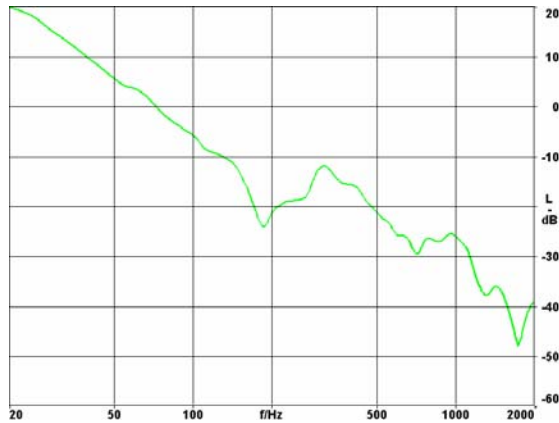
Fig. 5: Example of an effective engine mount transfer characteristic acceleration a into for F for an engine mount in z-direction
