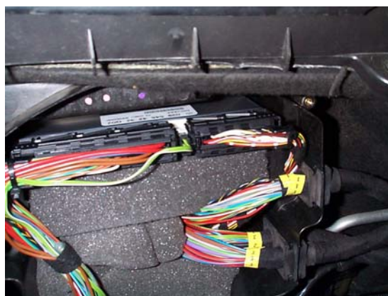
Figure 2: Fiche de raccordement du bus CAN
