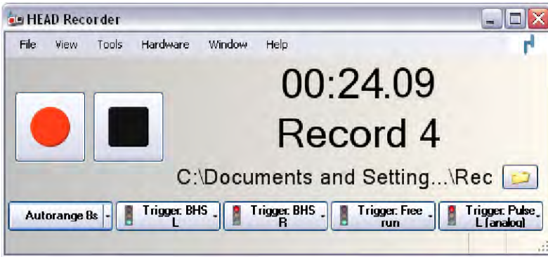
The main window of the HEAD Recorder with its large, easily accessible recording buttons and the five programmable buttons below.
