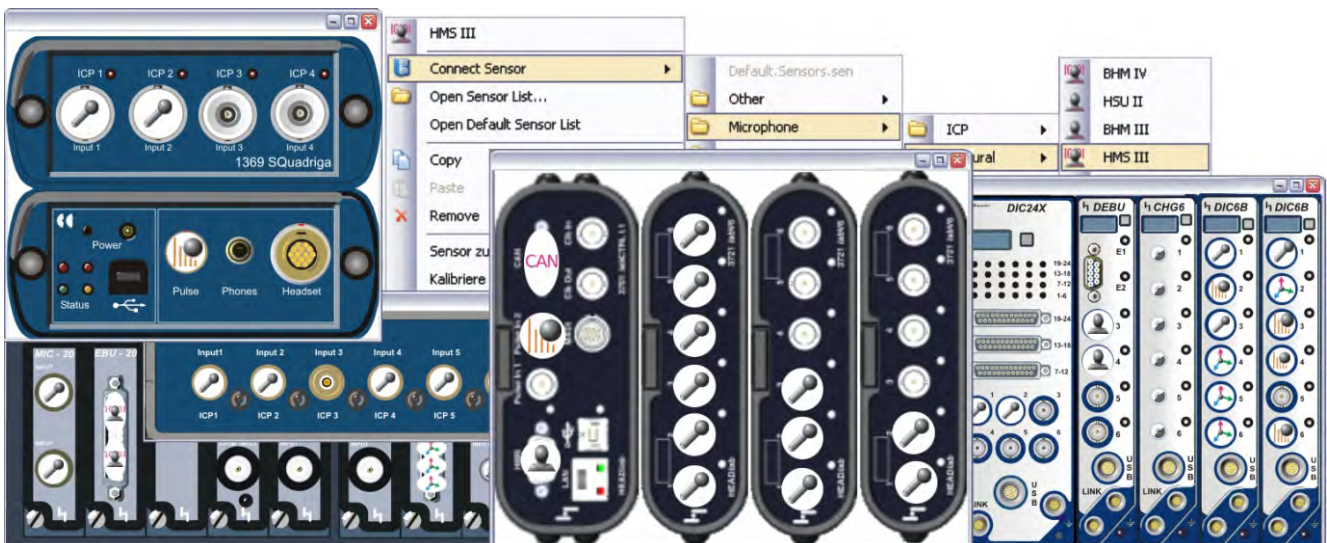
The front end view shows a photo of the connected front-end (HEADlab, SQuadriga III, SQuadriga, OctoBox+, DATaRec 4) and allows an intuitive connection of the sensors.
