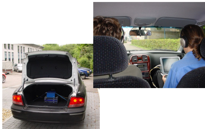
Figure 7: Mobile setup configuration of H3S installed in a roadworthy car
